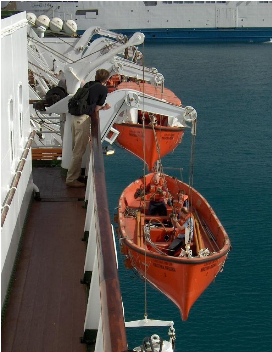
Figure 4. Lowering the lifeboats on M/S Kristina Regina (14.12.2008)
