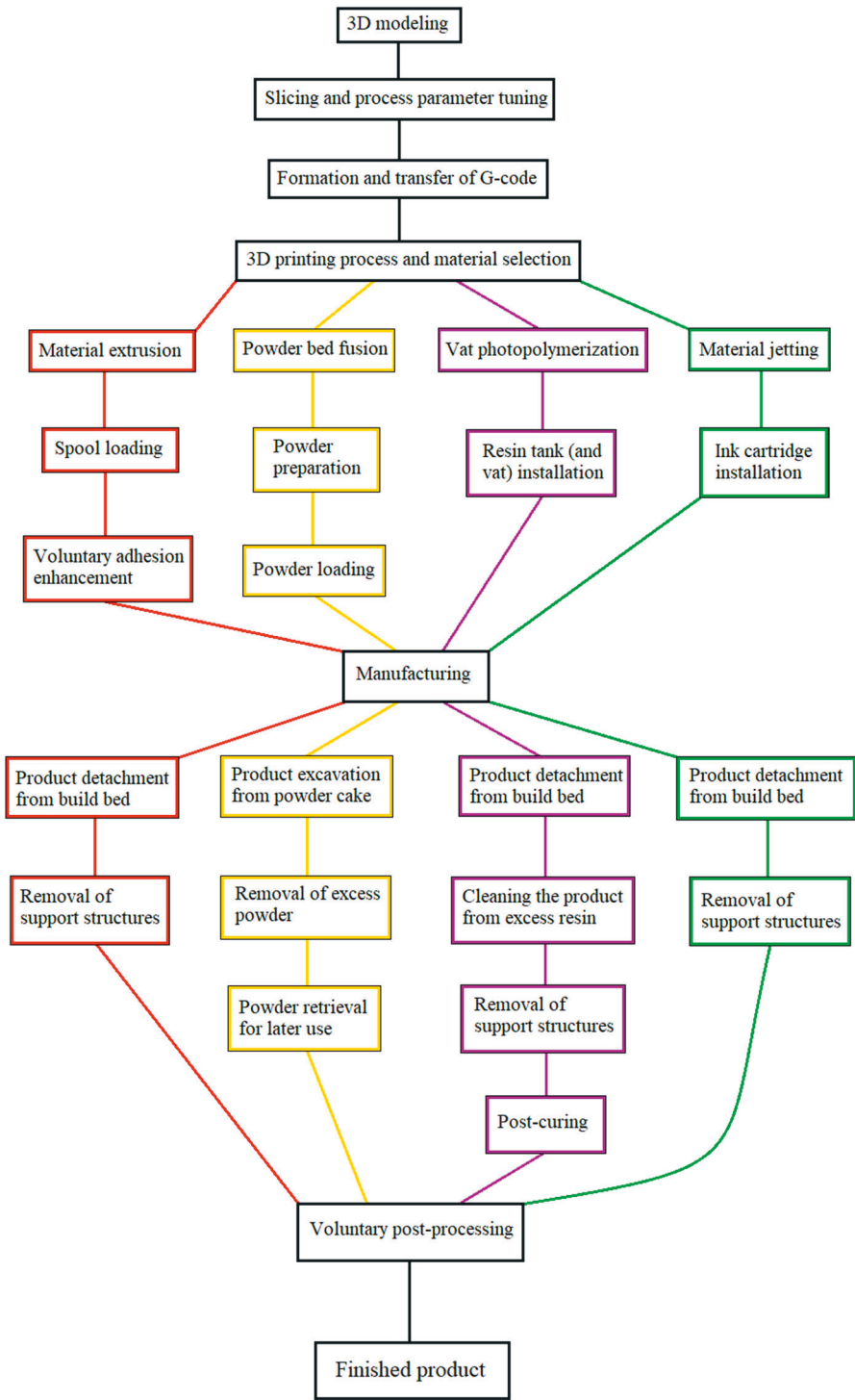
Figure 1. The additive manufacturing process flowchart.
