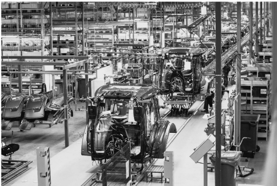
Fig. 2. Assembly line overview after development activities. In the figure, development activities like the product lifting table can be identified.
