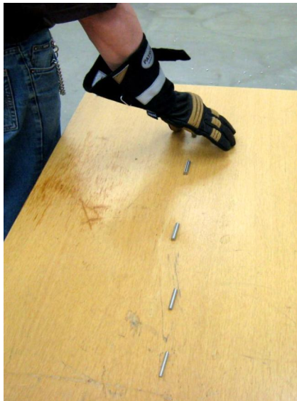
Figure 4. Finger dexterity tests with different gloves using five test pins
