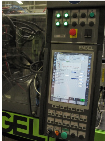
Figure 18. The control interface of an injection moulding machine in Fipak.
