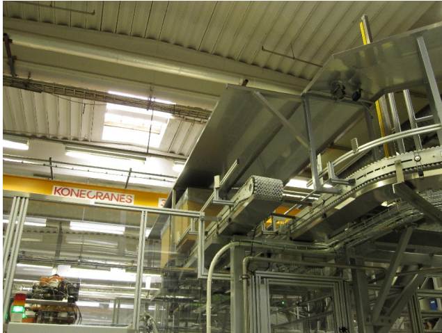
Figure 30. Transportation of empty and filled boxes to and from the packing robot in Fipak.
