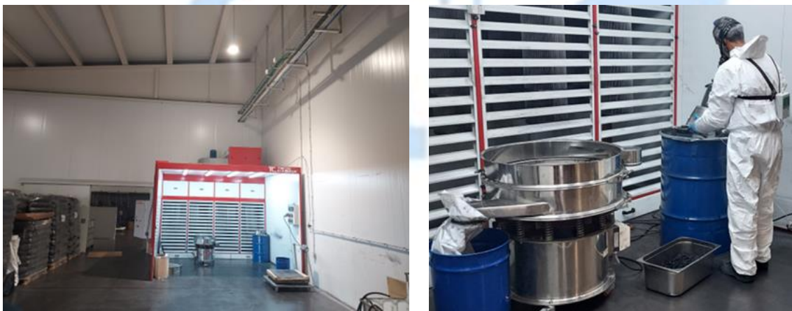
Figure 1. Filtration cabin in the manufacturing room, with the operator performing GO refining and packaging tasks inside.
