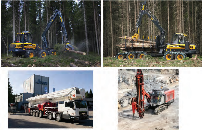
Figure 1.2. Top left: forest harvester, top right: forest forwarder, bottom left: truck mounted hydraulic platform, bottom right: drill rig. Pictures retrieved from www.ponsse.com , www.miningandconstruction.sandvik.com , and www.brnto.fi .
