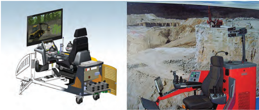
Figure 1.1. Working machine simulators: forest machine simulator (left) and drill rig simulator (right). Pictures retrieved from www.creanex.com .
