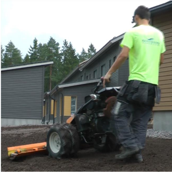
Bucher Elite 9 (E9 1-LH HSV, 6,7 kW) – sarvitraktori (163 kg) + 160 cm heilurijyrsin
