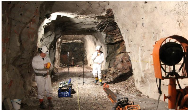
**Figure 8.1.** Overall view of the main practice drilling tunnel. The sound source was located at the far end of the tunnel and receiver locations varied along the tunnel.
