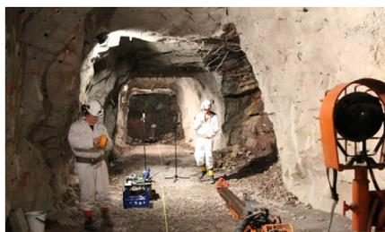
**Fig. 1.** Overall view of the main practice drilling tunnel. The sound source was located at the far end of the tunnel and receiver locations varied along the tunnel.
