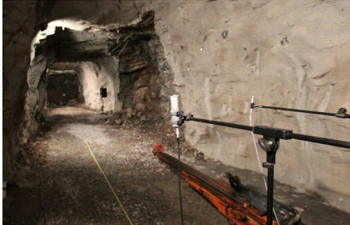
Figure 1: Overall view of the main practice drilling tunnel. The sound source was located at the far end of the tunnel and receiver locations varied along the tunnel. (Photo Otto Hedström)
