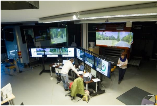
Fig 1. The simulator comprised parts of a real truck. The scenery was projected on screens covering the wind shields (SIMRAK, Tampere).
